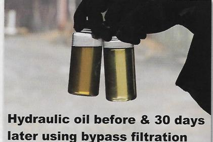
remove "ultra-fine" contamination and water that is normally missed by existing filters, dramatically extending the life of oil and the component it lubricates.
